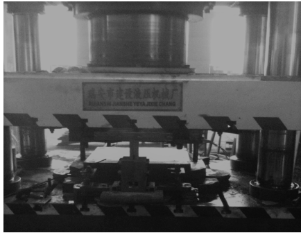
Fig. 3. Four column hydraulic press with die assembly
